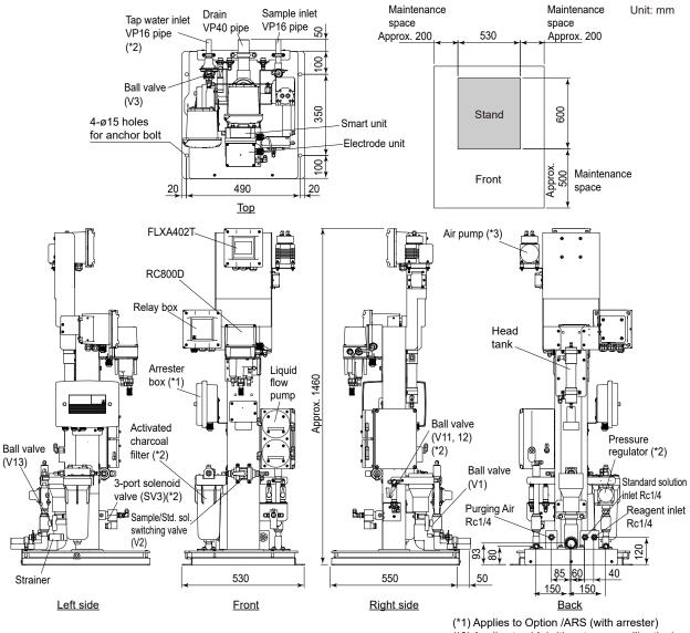
(\*2) Applies to -1A (with auto zero calibration) (\*3) Applies to -P $\square$  (pump for air purge)
